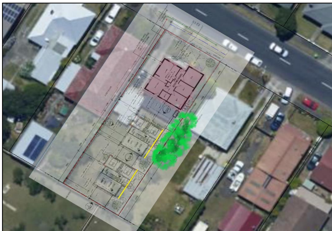
Figure 4. Screening vegetation at 34 Grove Road in excess of 5m in height (green) with the building line of the proposed shown as yellow.
