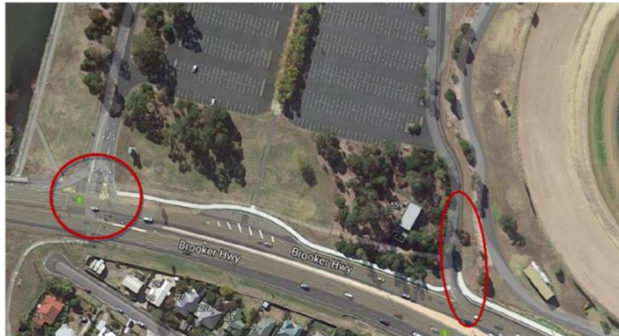
Figure 3: Showing the existing traffic signal-controlled access provision to the Wilkinsons Point site from the Brooker Highway in addition to the slip lane
